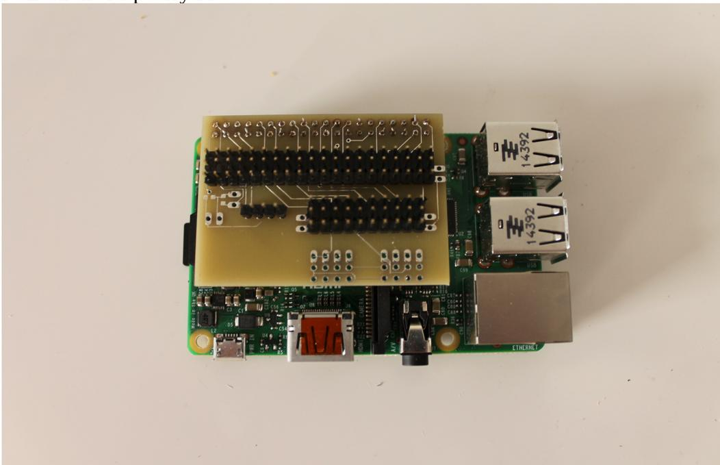
Power the PCB by plugging in the power cable and switching on the power switch
